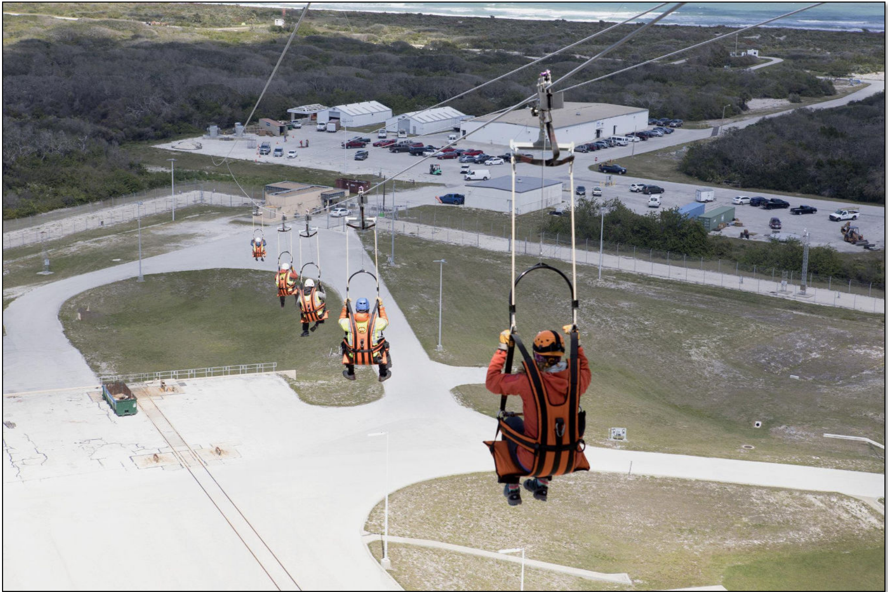
Test of a space shuttle zip line escape system for NASA astronauts. Credit: NASA. (Image from: https://www.space.com/36344-zip-line-emergency-escape-system-astronauts.html ).
