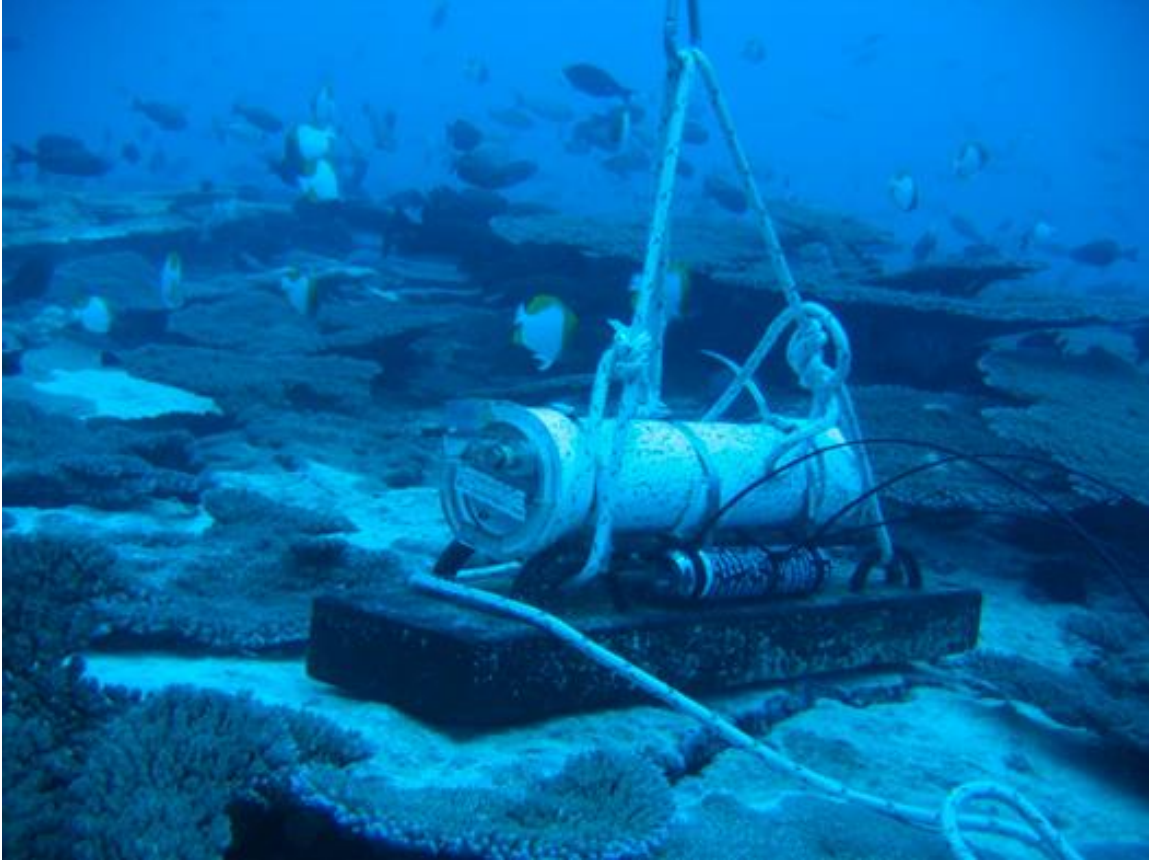
Figures 2 and 3: The Hawai'i Institute of Marine Biology uses Ecological Acoustic Recorders to study coral reefs. The devices are placed at different depths, depending on the kinds of sounds they are hoping to detect. (Images: NOAA Fisheries https://www.pifsc.noaa.gov/cred/ear.php ).
