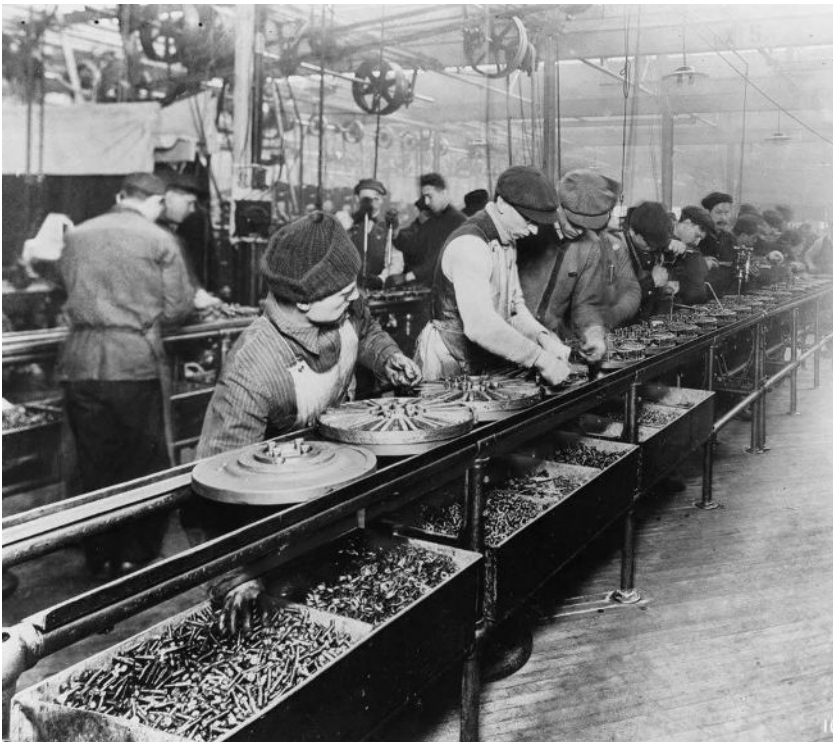
Figure 2: Workers at a Ford assembly line, 1913. Each worker completes just one step before the unfinished product moves on. (Image: Wikimedia Commons).
