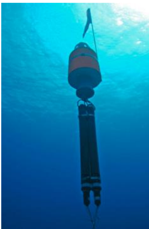
Figures 2 and 3: The Hawai'i Institute of Marine Biology uses Ecological Acoustic Recorders to study coral reefs. The devices are placed at different depths, depending on the kinds of sounds they are hoping to detect. (Images: NOAA Fisheries https://www.pifsc.noaa.gov/cred/ear.php ).
