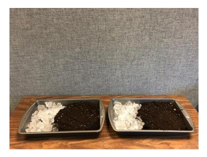
Place each house in a tray. Position them so that some of the house's base is over the ice, but one edge (or two stilt legs) rests on the ice-less soil. Pour hot water into the houses. You may want to fill a thermos with hot water so that you can refresh it once it cools.
